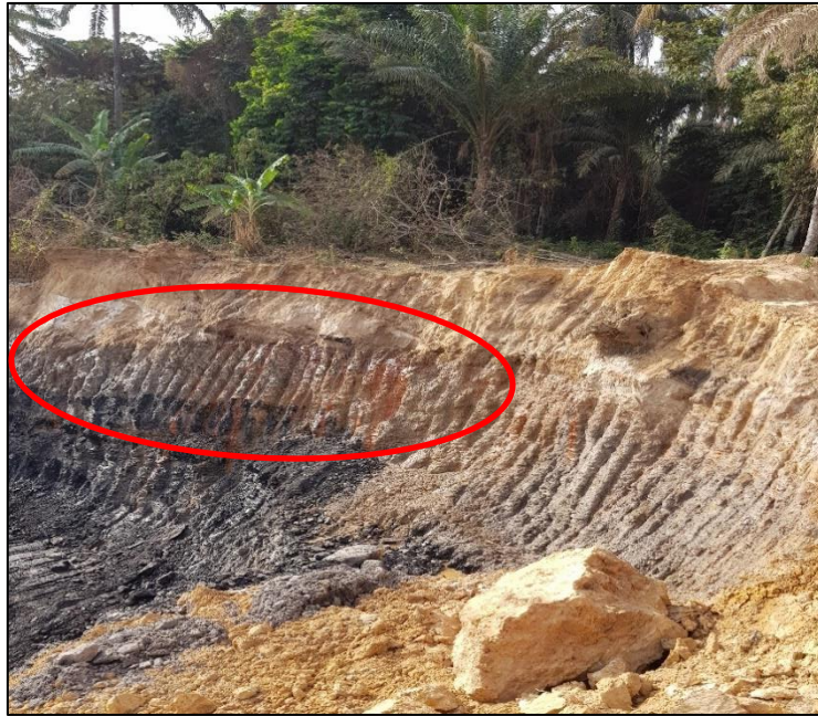
Figure 15: An example of interflow in the subsoil indicated by the red circle
