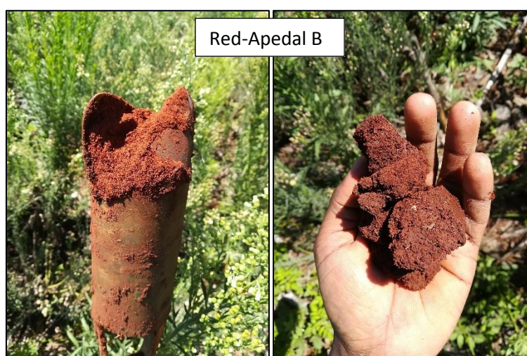
Figure 8: Representative photographs of recharge soils with deep, well aerated and free draining characteristics.
